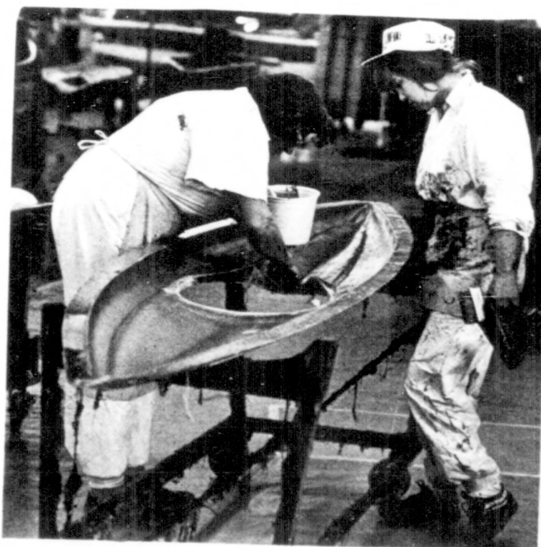
Old Town's fiberglass canoes and kayaks are the most lightweight and least expensive boats the company makes. Above, a worker cuts out a piece of fiberglass to fit the mold. Below, another worker touches up red paint on a kayak deck.
